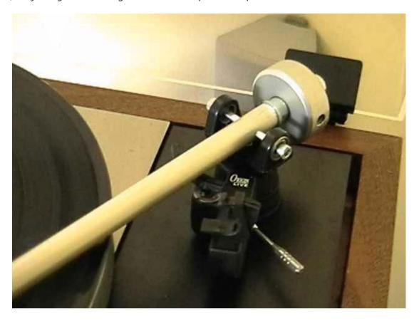
The arm lift mechanism is the same as can be found on Rega arms. It has a good positive feel and gently lowers the stylus into the groove. The arm clip was a little stiff at first but after a few weeks of use has freed up and is now fine.
